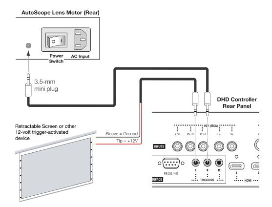
Figure 3-17. 12-volt Trigger Output Connections
